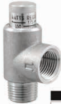
WATTS 530 - Calibrated pressure relief valve. Calibrated adjustment feature for setting valve to relief pressure. Adjustable range 50-175 lbs. All brass construction and stainless steel spring. Ideally suited as by-pass thermal expansion relief valve. 3/4".
