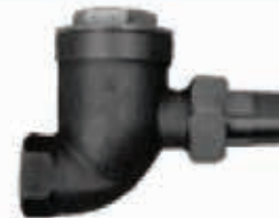
NO. 9C ANGLE STEAM TRAP - 1" pipe connections. Body, cap, nut and tailpiece are of high quality brass. Seat and thermostat are renewable. The thermostat, pin and seat are constructed of a non-corrosive alloy to give long life under actual service conditions. Stainless steel pin and seat available. Max 25 LBS.
