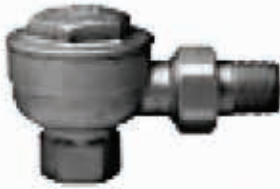
NO. 17C Low pressure traps. Max operating pressure 25 PSI. 1/2" x 1/2" Angle.
