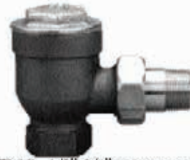
NO. 8C ANGLE STEAM TRAP 1/2"-3/4" pipe connections. Body, cap nut and tailpiece are of high quality brass. Seat and thermostat are renewable. The thermostat, pin and seat are constructed of a non-corrosive alloy to give long life under actual service conditions. Stainless steel pin and seat available. Max 25 PSI.
