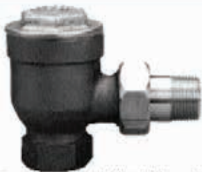
NO. 8 TRAP-1/2"x1/2" angle pattern. All bronze body, brass cap and unions. The thermostat is of a non-corrosive alloy to give long life under actual service conditions. The thermostat and seat are renewable. Seat and pin are stainless steel. Max 50 lbs.
