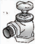
STEAM RADIATOR VALVE
