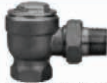
NO. 9 TRAP-3/4"x3/4" or 1"x1" angle pattern only. All bronze body, brass cap and unions. The thermostat is of a non-corrosive alloy to give long life under actual service conditions. The thermostat and seats are renewable. Seat and pins are stainless steel. Max 50 lbs.
