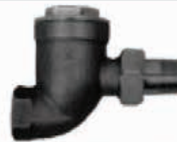
NO. 8C STRAIGHTWAY STEAM TRAP. 3/4" pipe connection. For radiator or convector locations which will not permit the use of an angle trap. Body, cap, nut and tailpiece are of high quality brass. Thermostat, pin and set are constructed of a non-corrosive alloy for maximum life under actual service conditions. Seat and thermostat renewable. Stainless steel pin and seat available. Max 25 LBS.
