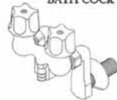
Bath faucet with cast brass body. Arms adjust from 2 1/2" to 8 1/2". Top handle. Chrome plated.
