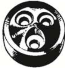
2 GPM Flow Restrictor. 3 variable orifices. Slips into threaded collar of shower head, cone pointing up. 2GPM @ 15 to 125 PSI.
